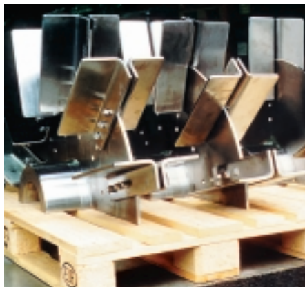
MAVA-Rut, segmented model for a 90 m 3 fermenter
